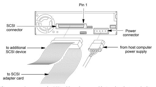
Connecting the SCSI cable and power cable (another device is the last Figure 2-3 device on the bus)
